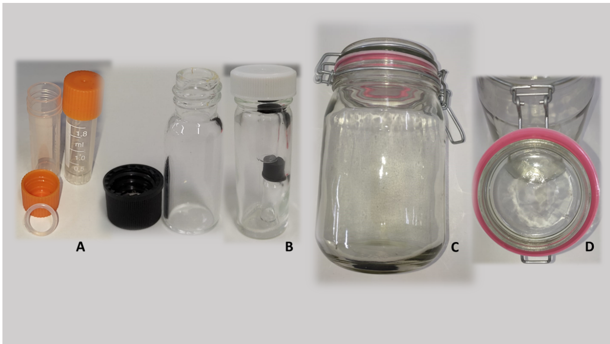
Figure 11. Examples of flasks for storing seeds. A. Flasks with silicon seals in the caps for seeds; B. Flasks for store few containing seeds, when possible a sachet of silica must be included in this larger flask; C. Large flask to storage of large amount of flasks, they must contain 2 cm of silica gel to maintain low relative humidity; D. Detail of the flask cover with the silicon seal.
